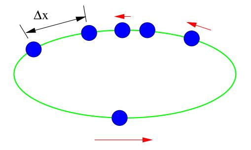
Velocity of cars v and position x, (in dimensionless formulation u, y). Bando model:
