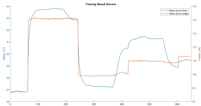
Figure 6: Graph of the training dataset. Where the blue line is the measured server temperature and the orange line is the server usage from the training data set.
