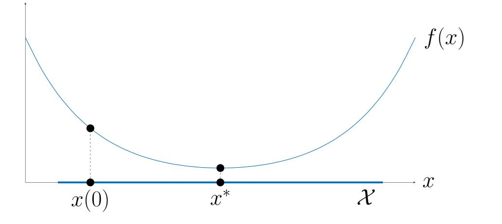
A distributed optimization algorithm is a numerical strategy for which a network of computers seek to maximize / minimize a cost f(x) that is defined (usually) as the sum of the local costs  $f_i(x)$  of the various computers, starting from a set of initial guesses  $x_i(0)$  and subject to the intersection of the local constraints  $\mathcal{X}_i$ . Importantly, in distributed strategies the various computing entities know only part of the available information.
