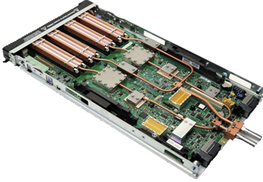
Figure 2: A typical liquid cooled blade server. The specific platform shown here is the IBM BladeCenter® QS22, it develops on a rectangular base that is 29mm wide, 245mm high and 446mm long and has all electronics with a power consumption above 3 Watts connected in the liquid cooling circuit.
