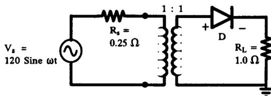
Fig. 4. Transformer Circuit Model
