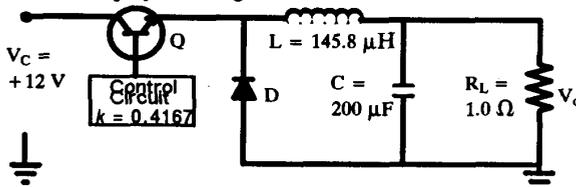
Fig. 1. Buck Regulator Circuit
