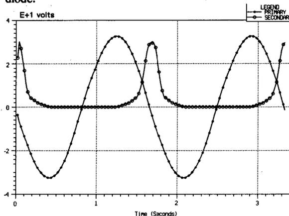
Fig. 7. Primary Voltage and Secondary Load Voltage
