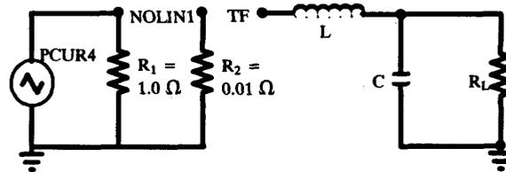
Fig. 2. Finite Element Circuit Model
