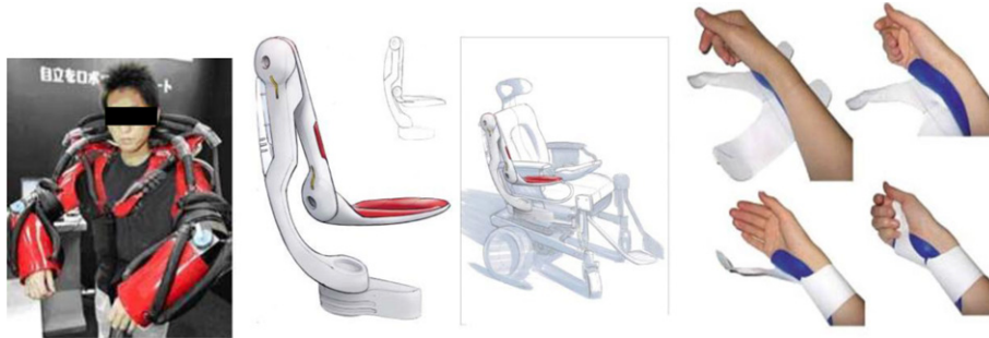
Fig. 4. An existing powered orthose (left), our design (center, here mounted on a wheelchair) and the “glove” control interface (right).
