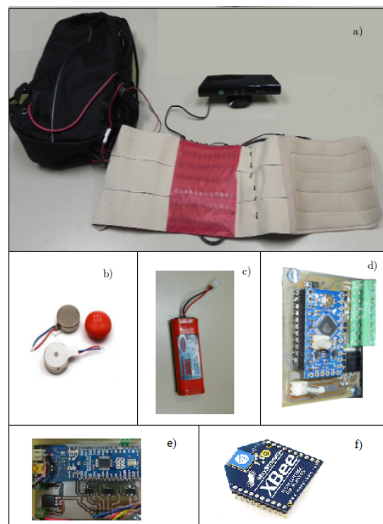
Figure 2. Hardware of TSIGHT, a) Kinect and waistband, b) Vibrotactile actuators, c) Battery, d) Slave I 2 C power module, e) master I 2 C module and f) XBee wireless device.
