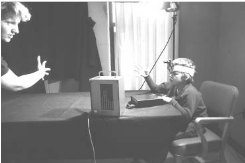
FIGURE 1 Child reproducing perceived image of a teachers hand as displayed on a modified Optacon. The tactile image is picked up with one finger statically placed on the 6 \times 24 vibrotactile array. LED monitor in foreground is visual representation of active pattern on the tactile display, which is obtained by the child's head-mounted camera.
