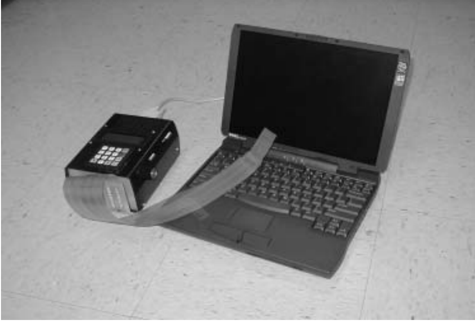
FIGURE 2 TDU-1 with 144-point tongue array & laptop PC.
