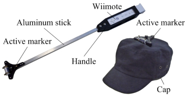
Fig. 2. Virtual augmented white cane with Wiimote and a cap with an active marker of accuTrack 500.
