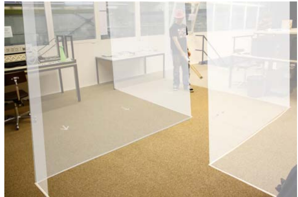
Fig. 1. Example of a virtual corridor invisible to the subject. The subject navigates in an empty room and receives vibrotactile and audio feedback in function of the distance to the virtual walls.
